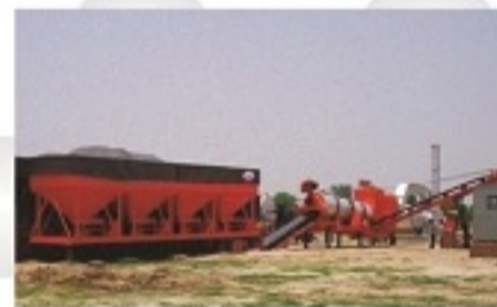
Asphalt Plant (Drum Mix)
